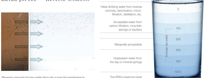
Reverse osmosis forces water through a special membrane to remove contaminants
